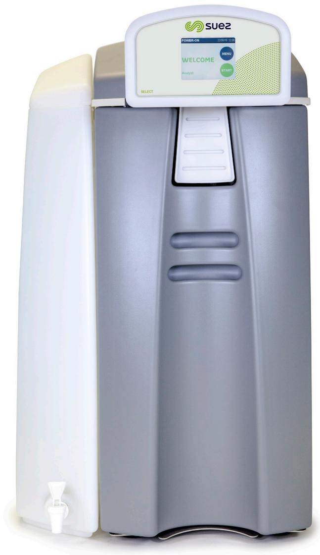
The Select Analyst is a compact unit ideal for laboratory use, delivering a steady supply of  $> 1\text{M}\Omega\cdot\text{cm}$  pure water for laboratory tasks using carbon pre-treatment, reverse osmosis and deionisation.
