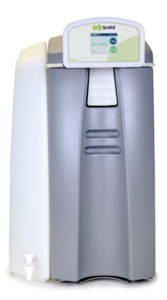
The Select edi 60 is a compact unit ideal for laboratory use delivering a constant supply of >1M $\Omega$ .cm pure water for laboratory tasks using activated carbon pre-treatment, double pass reverse osmosis, carbon dioxide membrane degassing and electrodeionisation technology.
